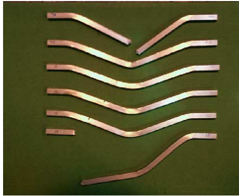
Fig. 15. Effect of notch location: Set 3 (nos. 10a, 10b, 10, 11, 12, 13).
