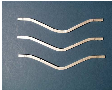
Fig. 19. Effect of notch location: Set 6b (nos. 44, 46, 48).
