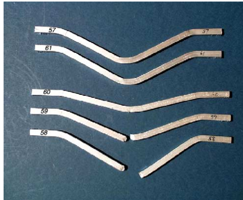
Fig. 10. Effect of notch's presence: Set 9 (nos. 57, 61, 60, 59, 58).
