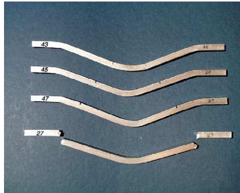
Fig. 18. Effect of notch location: Set 6a (nos. 43, 45, 47, 27).
