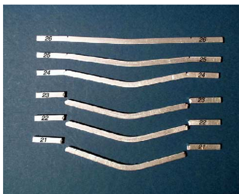
Fig. 12. Effect of increasing impact velocity: Set 7a (nos. 26, 25, 24, 23, 22, 21).
